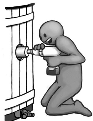
The Lead-in is connected to the plastic so that the rabbet of the sealing is on both sides of the barrel plastic and tightened securely.
