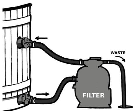
For winter and other times when the filter is removed, the return opening must be plugged with the cover/plugs included in the delivery. When the hot tub is not being used, the lead-through plug should be completely removed so that it doesn't get stuck on the lead-through part. During cold weather, the hot tub's valves (in older hot tub models) should be left half open even if the hot tub is empty, so that any water collected in the valves doesn't damage the valves when it freezes.
