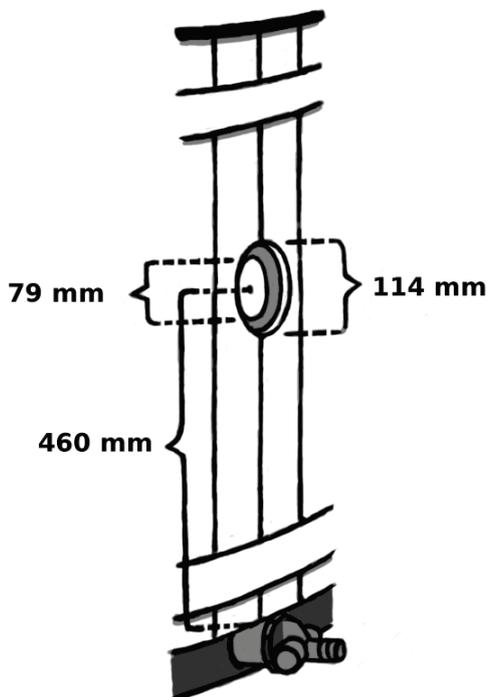
Installation of the Kirami grommet kit for a plastic barrel is very simple, you need to drill a hole just for a single inlet. A  $\varnothing 79$ mm hole needs to be drilled into the plastic itself and a  $>\varnothing 114$ mm hole into the wood panel at the same level. The hole in the upholstery needs to be bigger in order to tighten the inlet and to have enough space to rotate the components into position.
