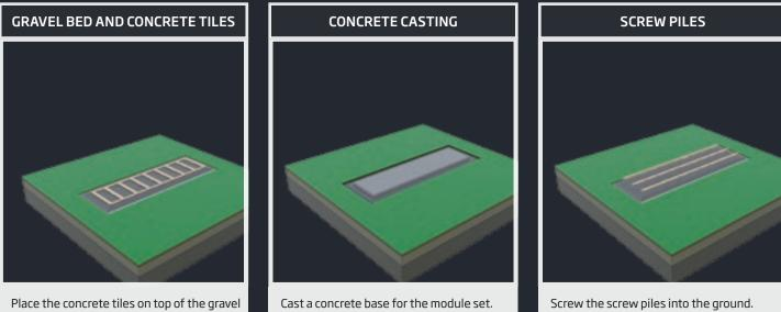
Screw the screw piles into the ground. Attach horizontal joists to the screw piles. Ask an expert which screw piles are suitable for your ground type.
