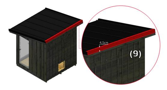
17. Finish by attaching the **end flashing (9)** to the back of the sauna with the **roofing screws (16).**
