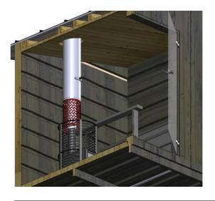
**4.** Place the basket for stones around the connecting pipe and fill it with smaller stones.
