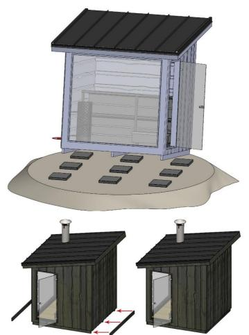
When the sauna has been lowered to its final location and the straightness has been checked with a level, attach the skirting boards to the front and the back of the sauna using terrace screws (12).
