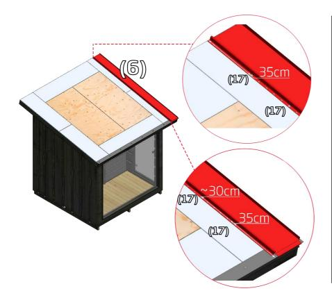
7. Start attaching with the roofing sheet, start piece (6) using wronic screws (17). Folded end of the sheets need to be located in front of the sauna. Recommended distance between the screws is 30cm but first and last screw is good to be at least 35cm from front and back end. All the sheets have pre-drilled holes.
