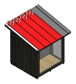
11. Attach rest of the wide roofing sheets (7) as shown in image 10.
