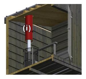
**3.** Install **chimney valve section (i).** It's recommended to place sauna stones after this.
