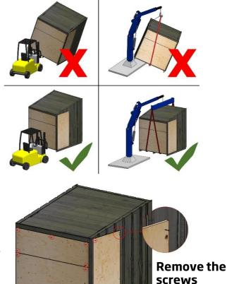
The sauna is delivered already assembled except for the roof, sauna heater, flue and door handle, which are installed by the customer. During transport, the sauna's own base acts as the pallet, which means that the sauna can be placed directly on top of the foundation prepared by the customer. For transport, protective plywood sheets (attached with screws) have been placed around the FinVision sauna in addition to
