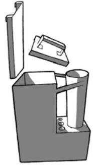
The SIDE, CUBE, and TUBE stoves have two grates and one solid L-shaped iron. They are installed on the stove brackets as indicated in the picture. The L-shaped iron should be the first edge turned upwards, this way it works as a spoiler and it also keeps the firewood in better. These should always be in place when using the stove. (Picture on right)
